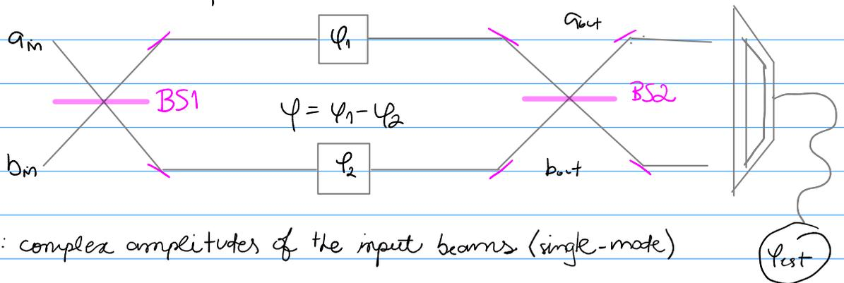
$a, b$ : complex amplitudes of the input beams (single-mode)
