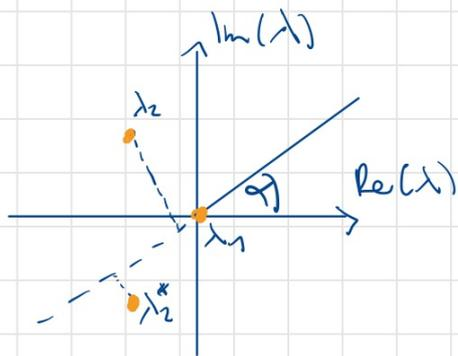
a positive  $\alpha$  moves eigenvalues in the upper-half plane closer to zero  $\Rightarrow$  they are less suppressed!
