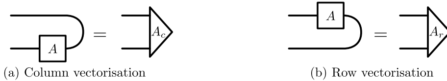
Figure 1.4: Vectorisation:(a) Column vectorisation, (b) Row vectorisation, and showing an operator that takes two legs, both of Hilbert space dimension d_{\text{HS}} and converts it to a single leg of dimension d_{\text{HS}}^2 . (c) converting a row vectorised vector a column vectorised vector by exchanging legs. Diagram adapted from Ref. [39].
