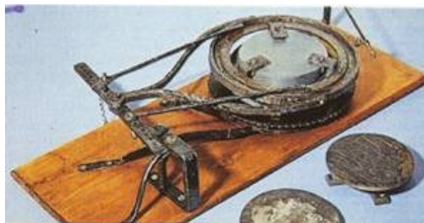
Figure 8. An early Herschel Mirror Polishing Machine. [P.D.]
