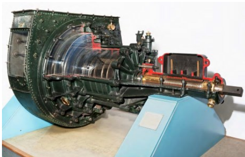
Figure 19. Turbinia's Original (1894) Radial Flow Turbine. [P.D.]
