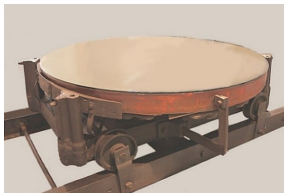
Figure12. The 6-foot Mirror on its Travelling Carriage. [P.D.]
