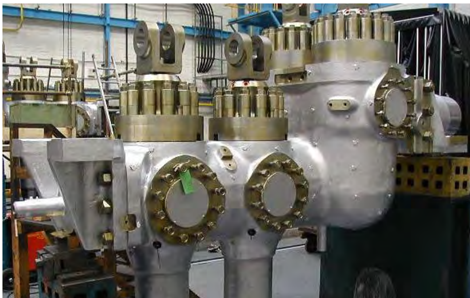
Fig.156 Cast 10 CrMoV HP steam chest manufactured in 2000. Since the expansion coefficient of 10 Cr steel was lower than the value for the Nimonic 80A studs retaining the valve covers, austenitic sleeves were fitted under the capnuts to compensate. The small pipes beneath and at the end of the chest were prewarming connections for fast starting.
