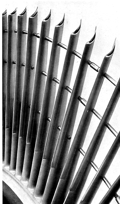
Fig.99 Hollow last stage blades used at North Tees C and Skelton Grange A
