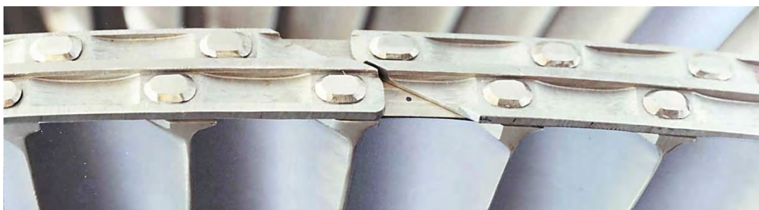
Fig.194 Revised coverband with obround tenons
