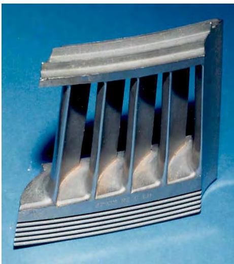
Fig.115 An IFR blade segment
