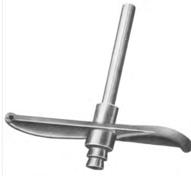
Fig.2 De Laval's Hero turbine of 1883 used to drive cream separators. [3]
