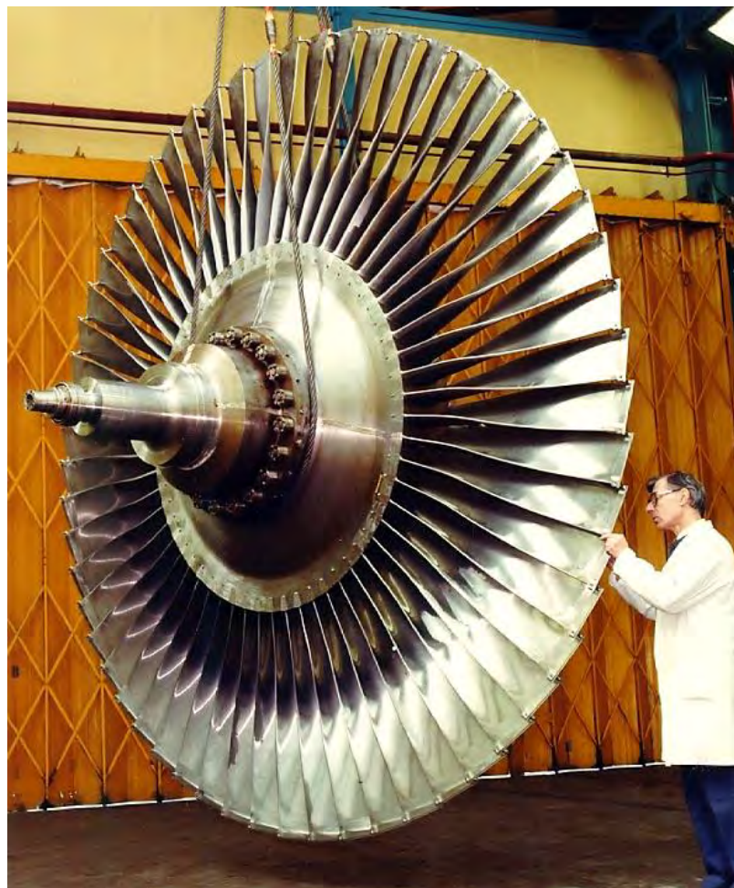
Fig.218a 1070 mm long high twist last stage LP blade with a curved side entry root fixing, left , and fig.218b an assembled blade row on a vibration test wheel, right
