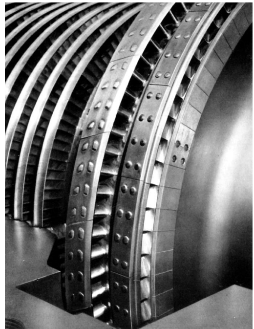
Fig.117 Cross-section through the HP turbine inlets Fig.118 Ferrybridge B HP turbine Curtis stage
