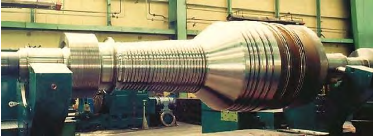
Fig.243 Dual heat treated 2 CrMoNiWV steel rotor for La Collette
