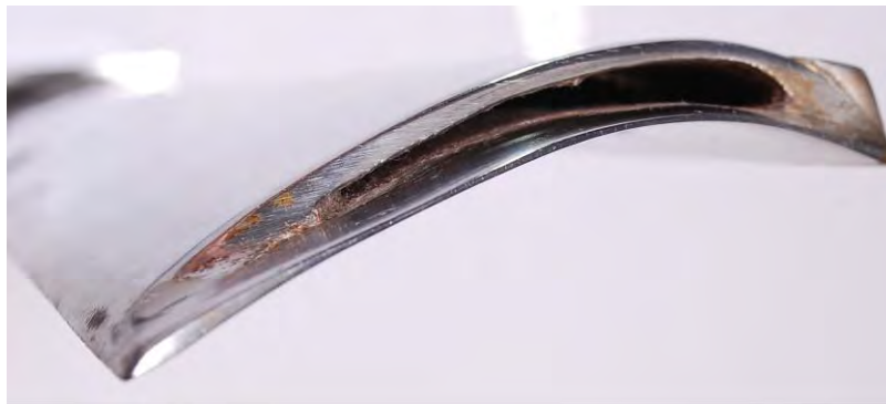
Fig.82 Close up view of the Dunston B blade showing the hollow aerofoil and the blunt-faced erosion shield attached to the leading edge, right hand side
