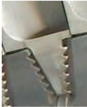
Fig.167 Parsons fir tree root fixing after modification
