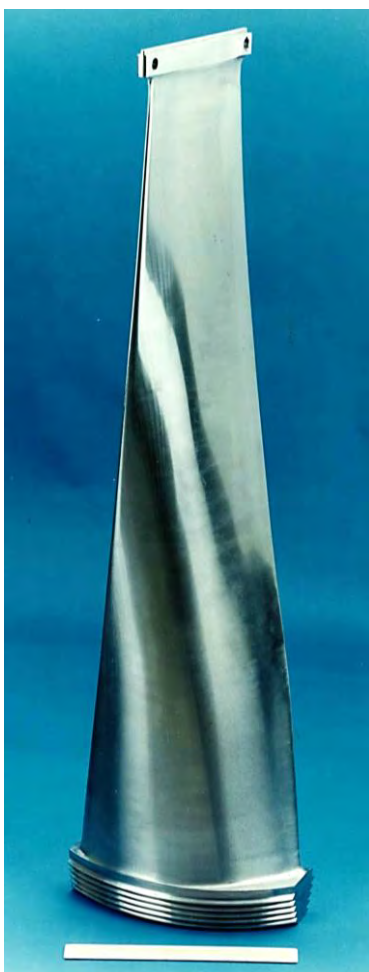
Fig.218a 1070 mm long high twist last stage LP blade with a curved side entry root fixing, left , and fig.218b an assembled blade row on a vibration test wheel, right
