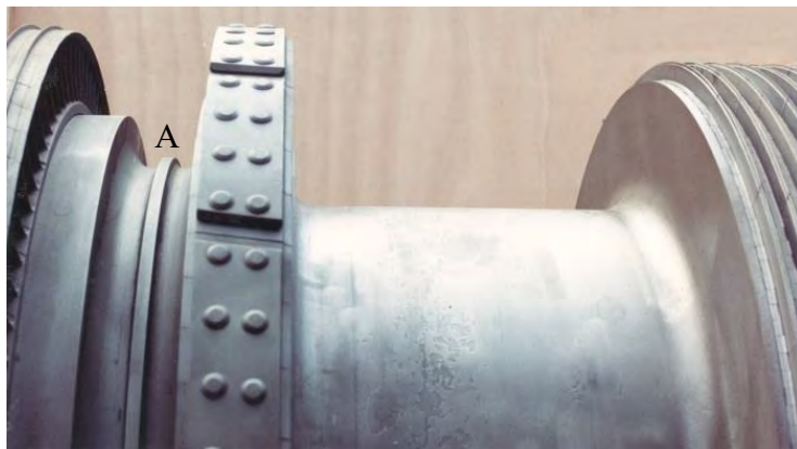
Fig.222 Comparison of the HP turbine rotor inlet geometry for Drax, left , and Lamma Island, right . The feature marked A was specified in the 1960s to allow the creep growth of rotors to be measured.
