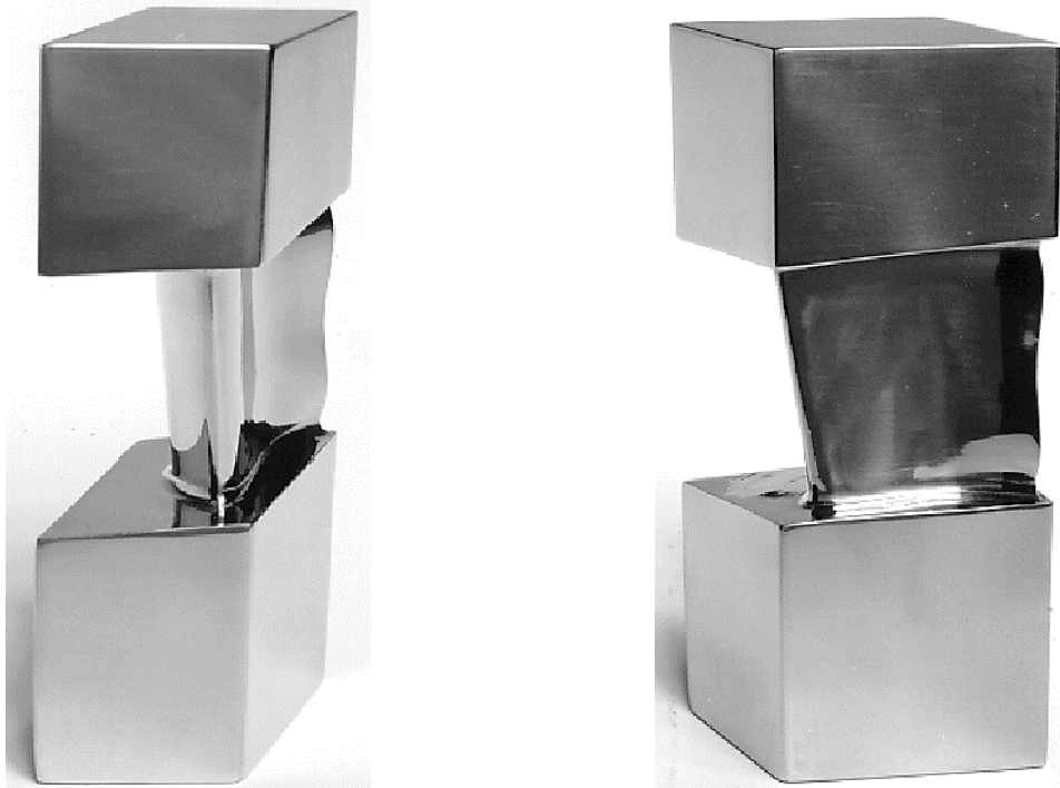
Fig.232 A 3D reaction blade using ‘end bends’ in the trailing edge to increase the blade throat opening close to the hub and tip to suppress flow vortices
