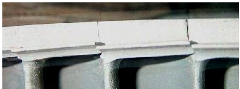
Fig.116 Shroud lifting known as 'crocodile's teeth'
