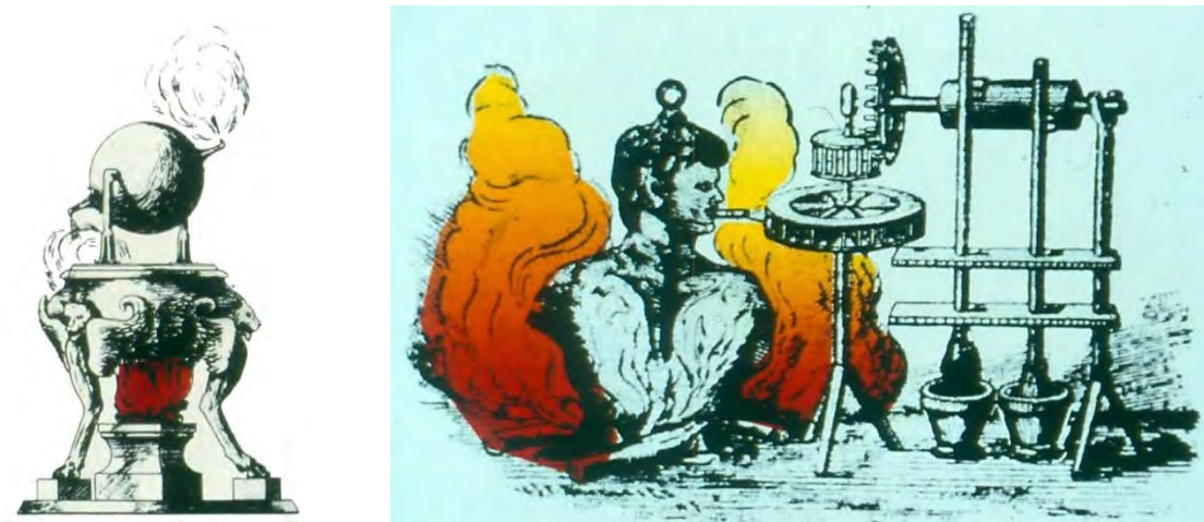
Fig.1a Hero's aeolipile or reaction turbine, left , and fig.1b Branca's impulse turbine, right
