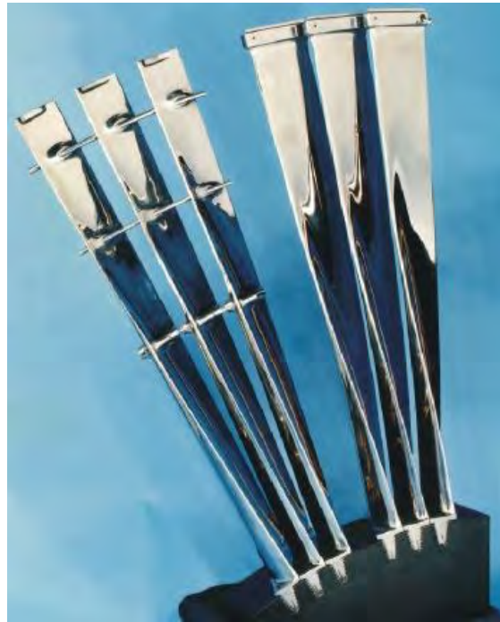
Fig.168 Comparison between the original 500 MW last stage blades, left , and high efficiency, high twist blades, right
