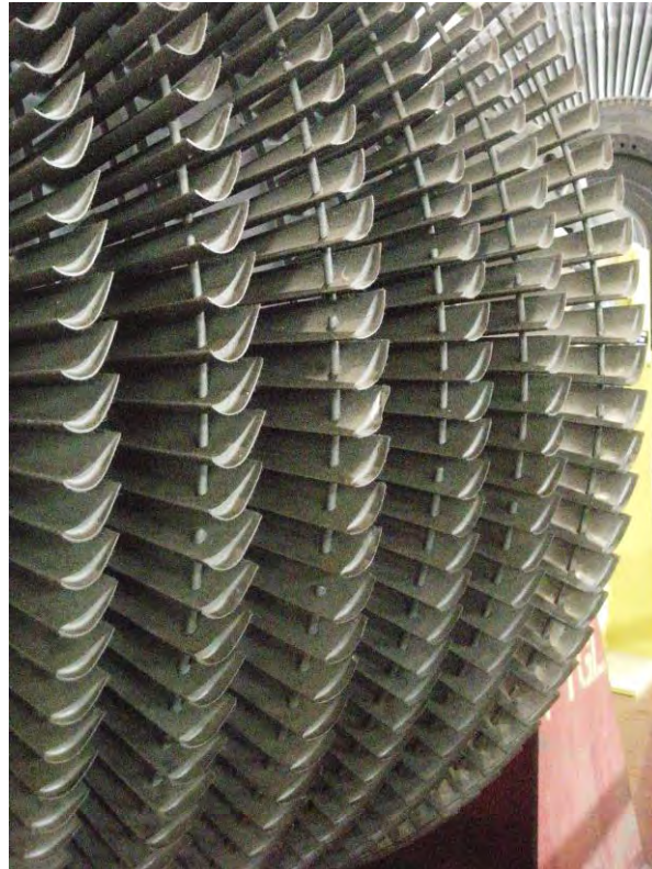
Fig.204 Pickering HP turbine blading stages 9 to 14 after 35 years' service
