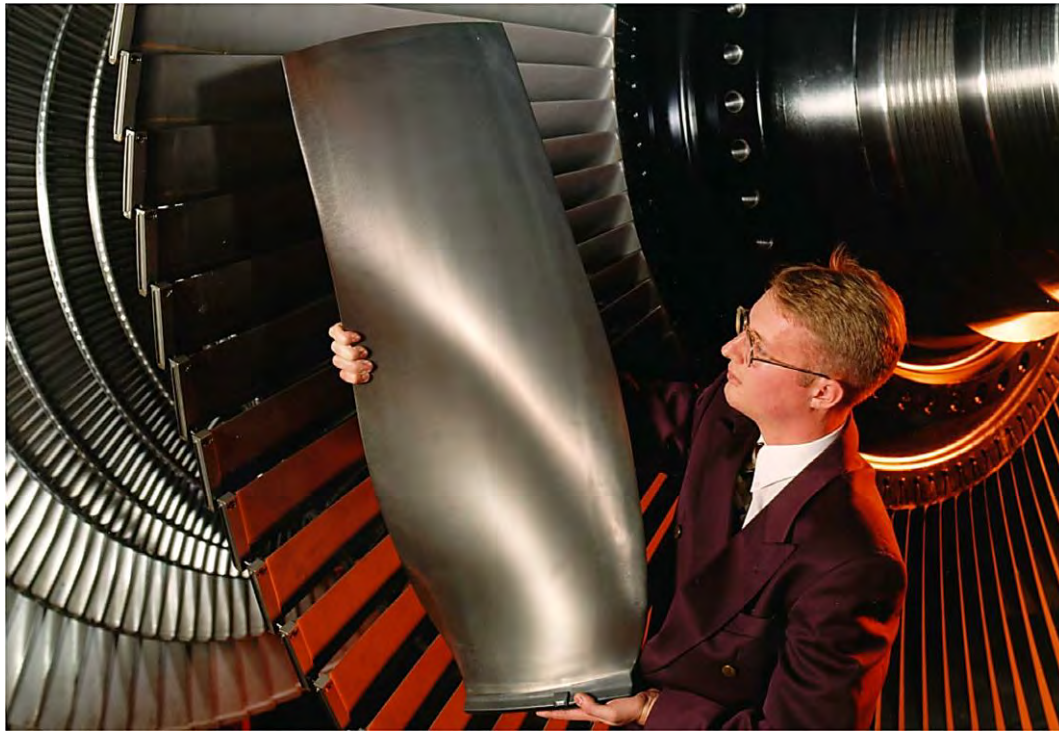
Fig.237 A hollow titanium fan blade from a Trent aero-engine compared with a typical Parsons steel LP last stage blade
