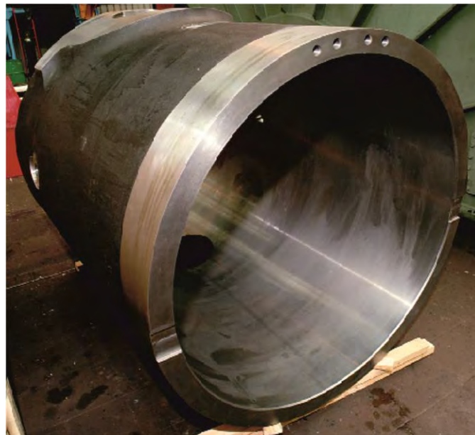
Fig.187 Drax HP turbine barrel or middle casing
