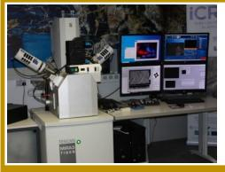
New improvements have been made to the SEM instrument in the iCRAG Lab at TCD. The SEM has Colour CL, BSE, in-lens detectors and a Deben tensile stage completed the package. An EBSD detector will be added in the near future. More photos and information about the installation can be found here.
